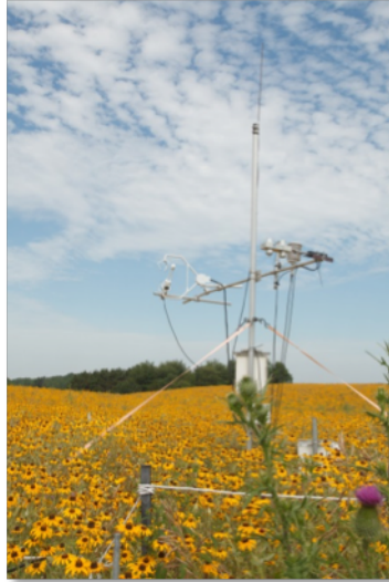
Figure 3.2: Eddy covariance tower at scale-up fields (see Figure 3.3) used to estimate C balance of annual and perennial cropping systems.
